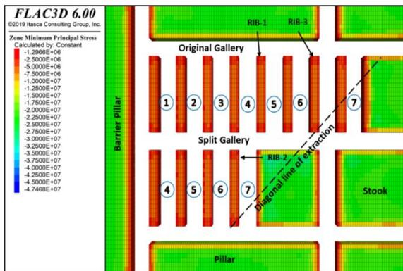
**Figure 3** Principal stress distribution on rib and coal pillar during depillaring
