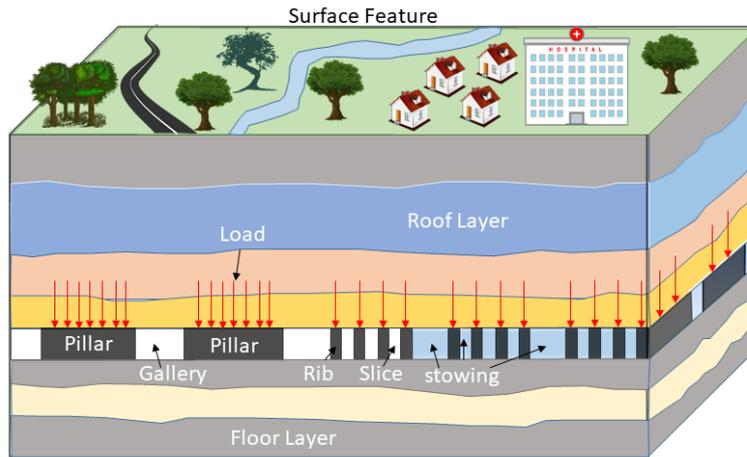
**Fig. 1.** Conceptual image representing backfilling in goaf to protect surface feature
