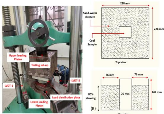
**Figure 5** Experimental set up for compression testing with sand stowing
