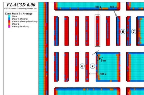
**Figure 4** Propagation of failure zone in rib and pillar during depillaring
