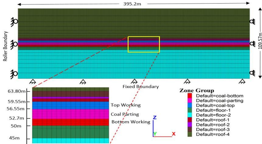
**Figure 2:** Three-dimensional model preparation in FLAC3D
