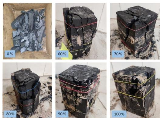
**Figure 6:** Rectangular coal sample failure state after compression
